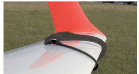
Bug wiping systems are based on a nylon string, which is pulled along the leading edge of the wing, scraping off the remains of the bugs. Pictured above is the cleaning procedure from the parking position to the position at the wingtip showing the 'MP' Mückenputzer (streckenflug.at)
