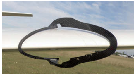
Bug wiping systems are based on a nylon string, which is pulled along the leading edge of the wing, scraping off the remains of the bugs. Pictured above is the cleaning procedure from the parking position to the position at the wingtip showing the 'MP' Mückenputzer (streckenflug.at)
