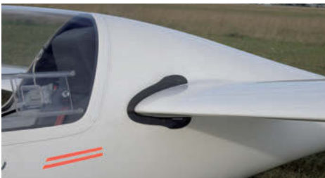
Bug wiping systems are based on a nylon string, which is pulled along the leading edge of the wing, scraping off the remains of the bugs. Pictured above is the cleaning procedure from the parking position to the position at the wingtip showing the 'MP' Mückenputzer (streckenflug.at)
