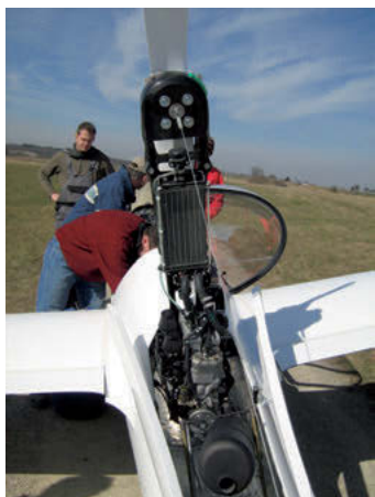
The engine installation in the Nimbus 4DLM was developed by Walter Binder
