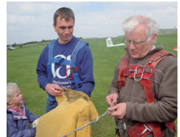
Graeme is holding Peter's jacket with burn marks around the collar. Peter is holding a section of the aluminium steering rods that buckled and twisted from the powerful magnetic force of the lightning
