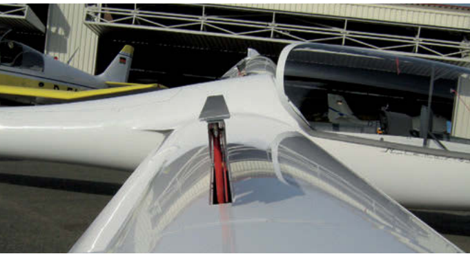
The two-bladed Schempp-Hirth airbrakes are efficient and connected via a gas spring strut to the inner flap section to compensate for the loss of lift caused by the airbrakes
