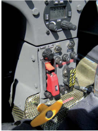
In the socket of the front instrument panel, a protected switch permits handing engine control over to the rear seat. The second one serves to operate the retraction manually in case of an emergency
