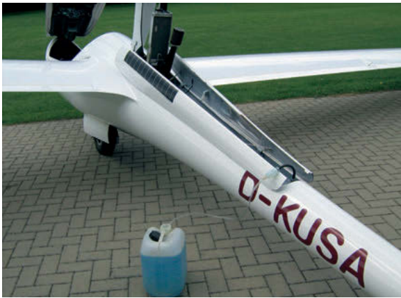
Refuelling is easy with the built-in fuel pump
