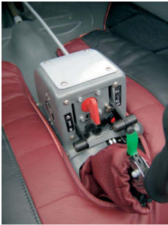
Throttle (left), propeller stopper (right) and starter button (underneath the propeller stopper) are placed in the socket of the instrument panel
