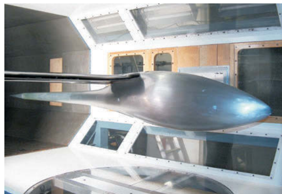
Figure 24 Wind tunnel model of the Mü-31 wing-fuselage combination
