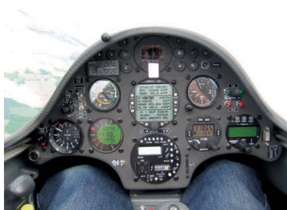
The engine control instrument is placed central in the bottom of the instrument panel, the engine main switch left
