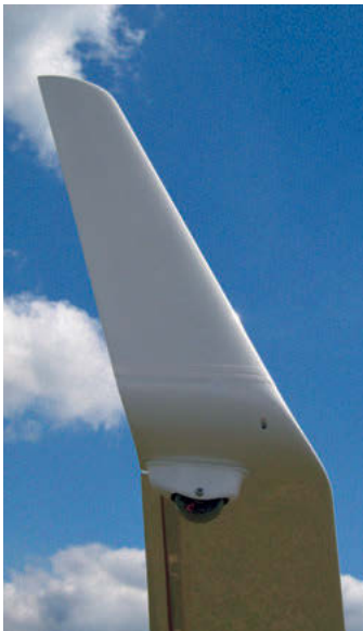
The winglets fit to both outer wings, the small wingtip wheels will be larger in serial production
