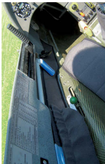
In the front cockpit, flap lever (black), airbrake lever (blue) and trim button (green) are placed ergonomically, the cable release (yellow) a bit too low
