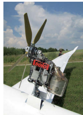
The Oehler solo 2350 sustainer drive
