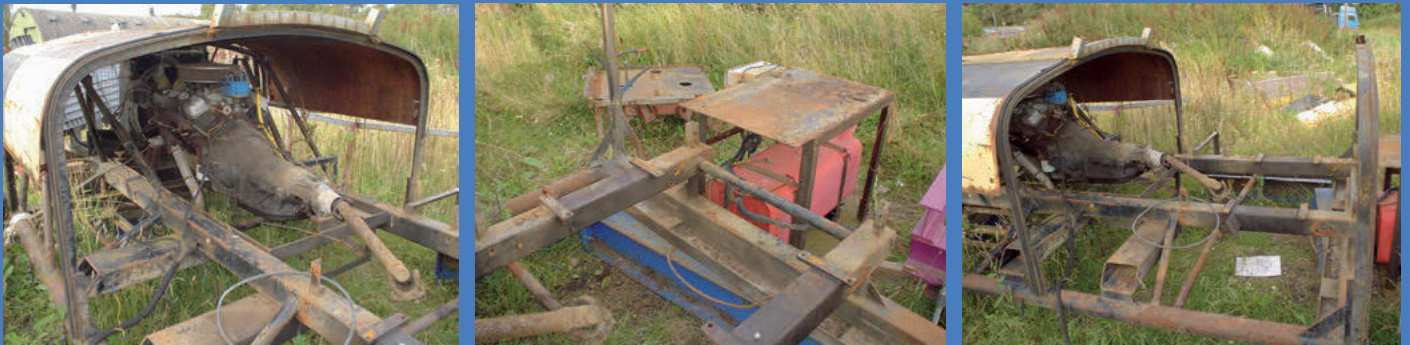
Skylaunch built a re-engineered winch for Surrey Hills GC using components refurbished to a nearly-new condition (Russell King)
