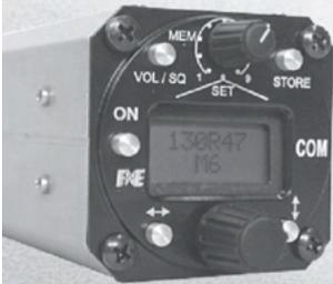
**ATR500 Radio** Entry level 57 mm radio with easy operation via 2 line LC-Display 9 memory frequencies, Auto TX off after 2 mins Power supply: 10.5V - 14V price **£897.00 incl VAT**
