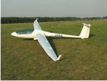
Sportline Aviacija's latest design with a completely new 4 piece wing developed by Krzysztof Kubrynski for the 18m class with a maximum All Up Weight of 600kg
