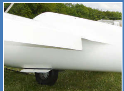
Above right: ASW 20C wing pitot connected to the blow holes
