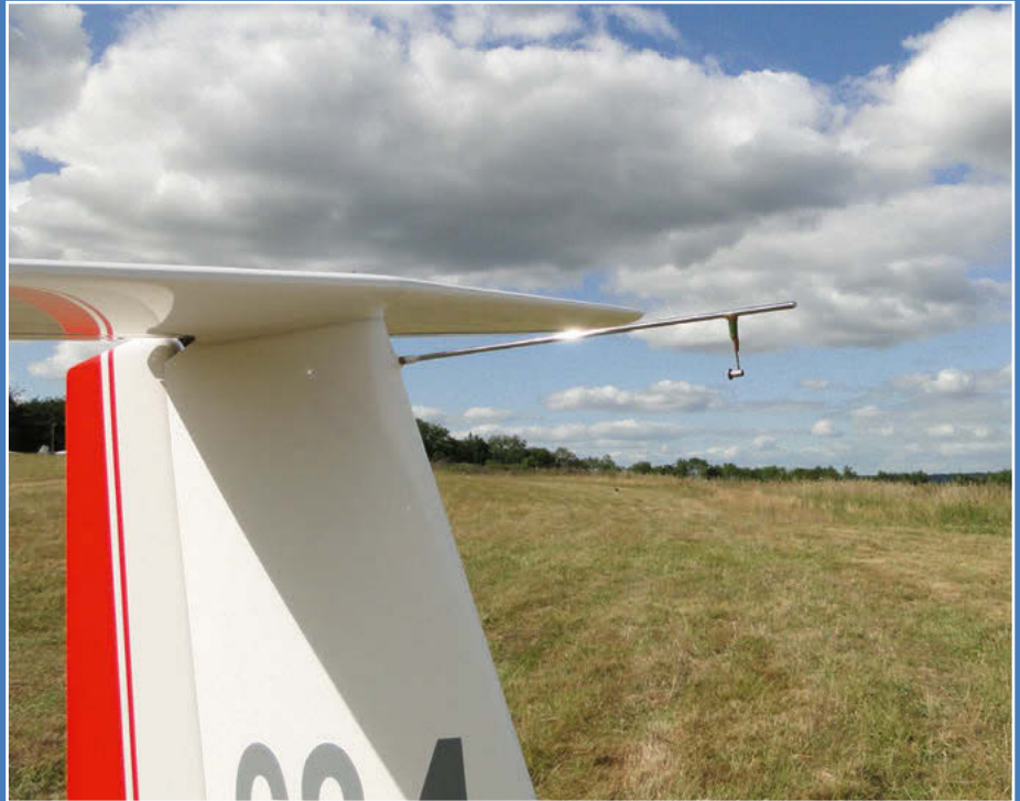
ASW 20C wing pitot, static and TE probe
