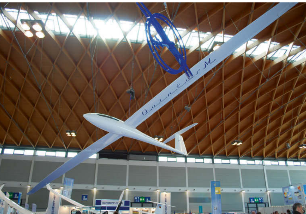
Lange Aviation's Antares 23E (above) shares its inner wing with the Schempp-Hirth Quintus M pictured below www.lange-aviation.com/www.schempp-hirth.com
