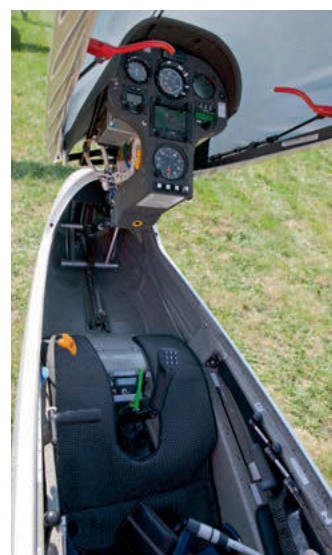
The cockpit of the LS10, familiar to most LS owners, with two water release knobs on the left-hand side and the large flap lever on the right (photograph by elfo.sk)
