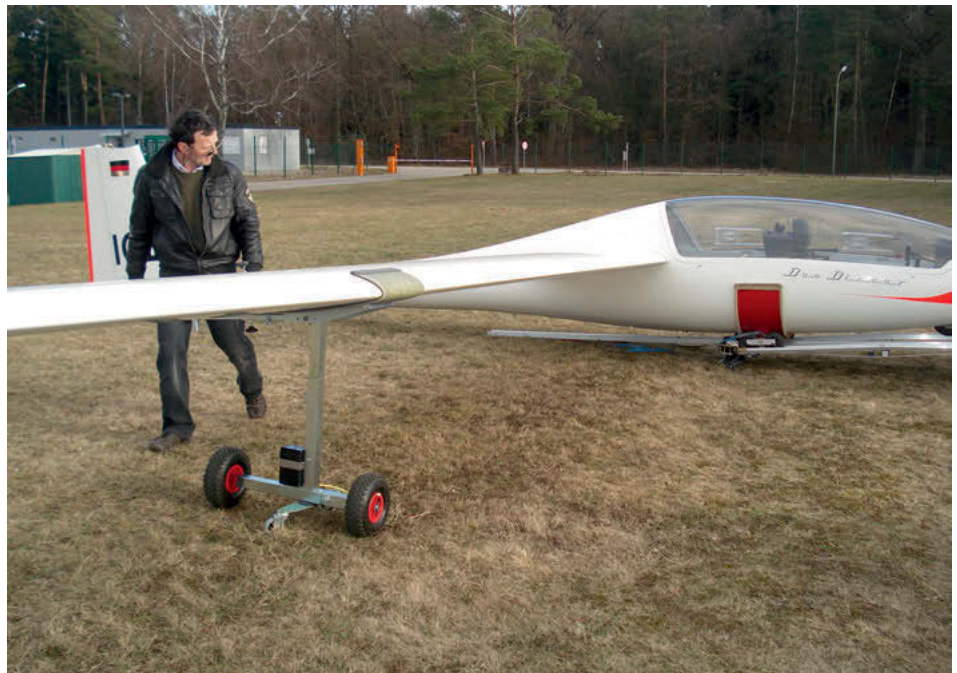
The Single Person Rigging Cart features a remote controlled electric drive system. It weighs 18kg and can be quickly disassembled into smaller components for storage in a trailer or car boot (photographs from Enstroj)
