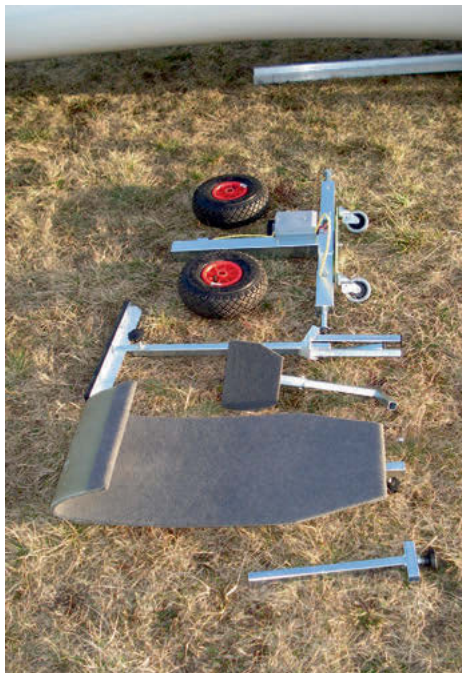
The Single Person Rigging Cart features a remote controlled electric drive system. It weighs 18kg and can be quickly disassembled into smaller components for storage in a trailer or car boot (photographs from Enstroj)
