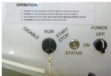
A simple start-up procedure involves plugging it in and turning a key (above). The computer power is pictured below (Keith Auchterlonie)
