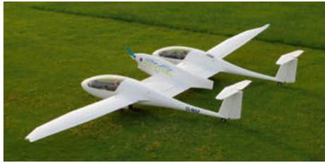
› This unusual electric airplane with room for four – the Taurus G4 – was Pipistrel's entry to the NASA/CAFE Green Flight Challenge on 25 September. It was built in just months, specifically for the competition, and is a test bed to develop a high-power electric propulsion system.
