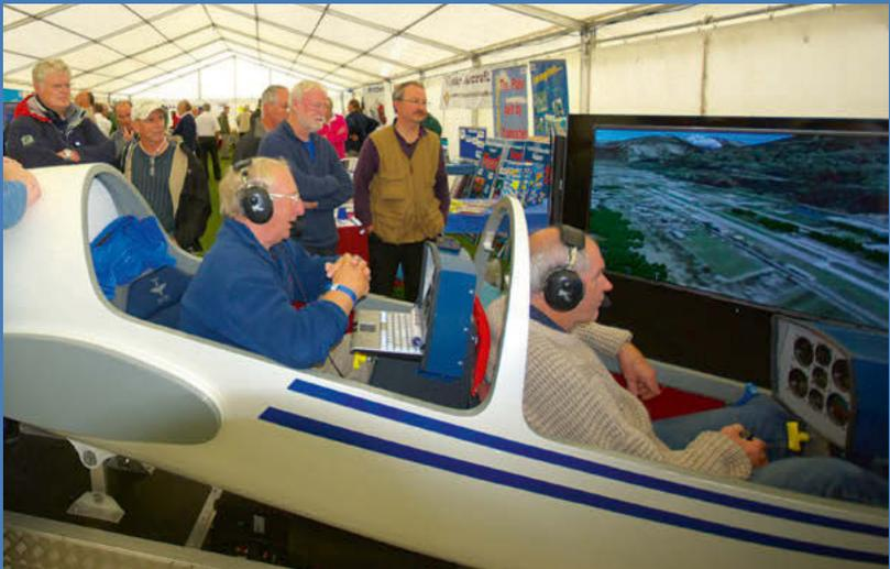
An easily viewable open cockpit, bright main visual displays and articulated side displays make it easier for bystanders to understand what is going on
