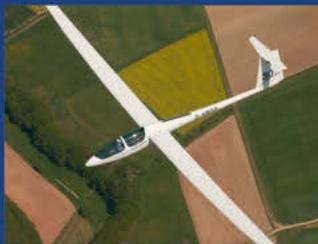
ASH30MI 2 seat open class self launcher auto controls
