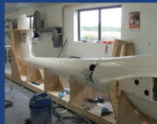
ASK21 in our Jig for fuselage repair
