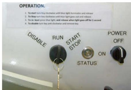
A simple start-up procedure involves plugging it in and turning a key (above). The computer power is pictured below (Keith Auchterlonie)
