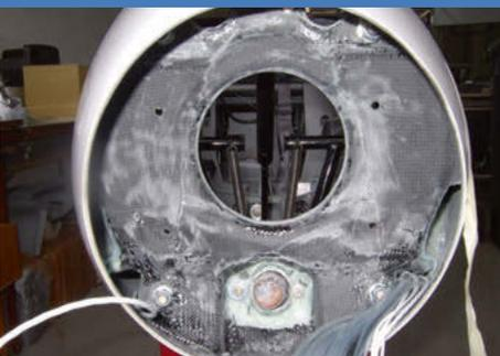
Existing bulkhead/pedal mount, exposed for motor mounting
