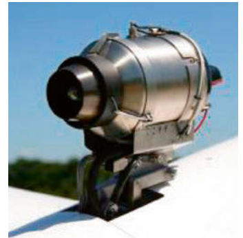
Proven Jet powerplant with over 600 made (Craig Lowrie)
