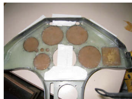
Infills bonded in with resin on a flat non-stick surface.
