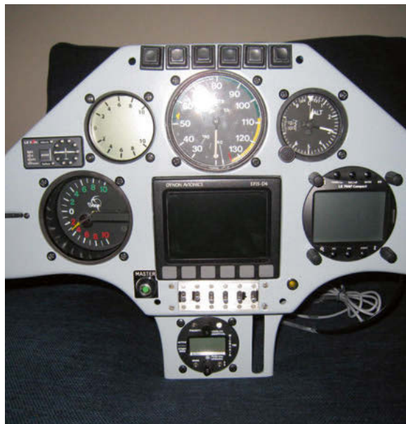
Instruments fitted and bench tested
