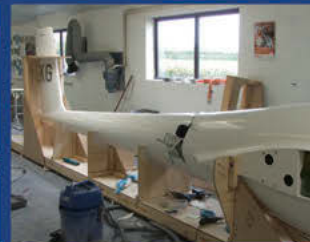
ASK21 in our Jig for fuselage repair
