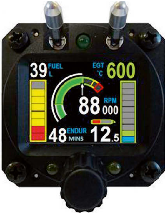
The Jet Display Unit (JDU) was developed specifically for the JS1-TJ
