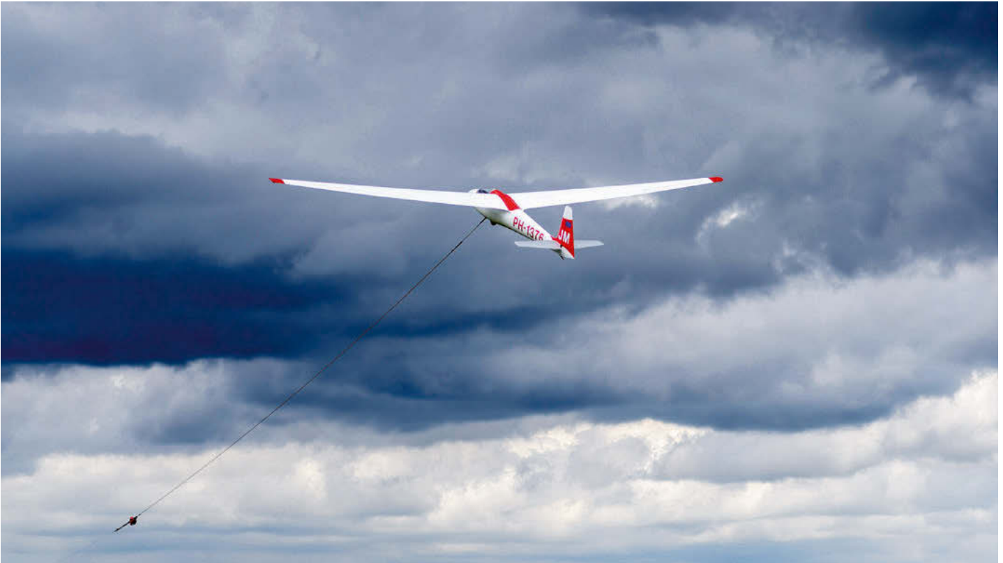
K-6E PH-1376 is winch launched at the Wenlock Olympian Gliding competition, held at the Long Mynd in July 2012 (Paul van der Zwan)
