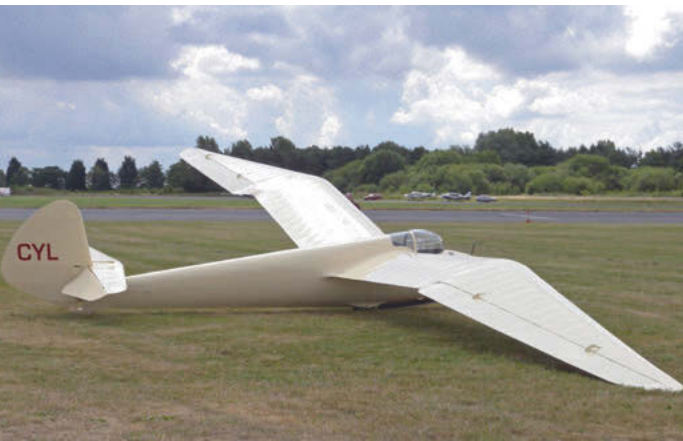
The Minimoa is one of the classic glider shapes of all time. Its design dates back to 1935 and you can see the influence of the birds within its features in both wing shape and gull wing dihedral (Martin Simons)
