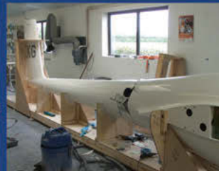
ASK21 in our Jig for fuselage repair
