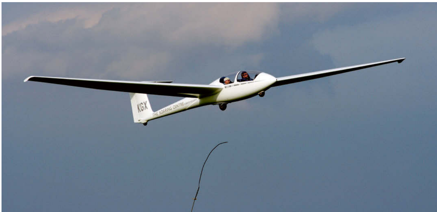
Cable back releasing after a launch failure (Mike Fox)
