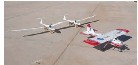
The 1/3-scale twin-fuselage glider that would be used to validate the flight characteristics of the Towed Glider Air-Launch Concept is pictured with its DROID tow plane on the ramp at NASA Dryden (NASA/Tom Tschida)
