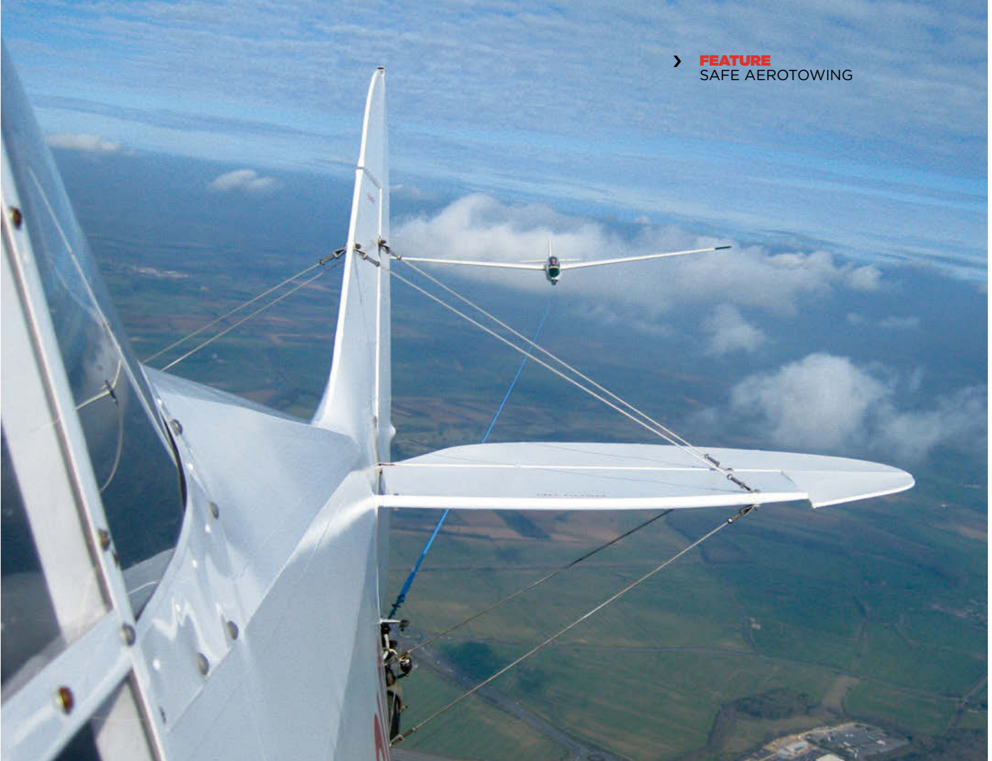
This photograph, which was taken from Banbury's Pawnee, illustrates a correct aerotow configuration (Robert Cronk)
