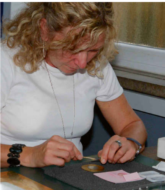
Left: production of spare part for diaphragms, and (above) calibration of airspeed indicators (All photographs courtesy of Winter Instruments)
