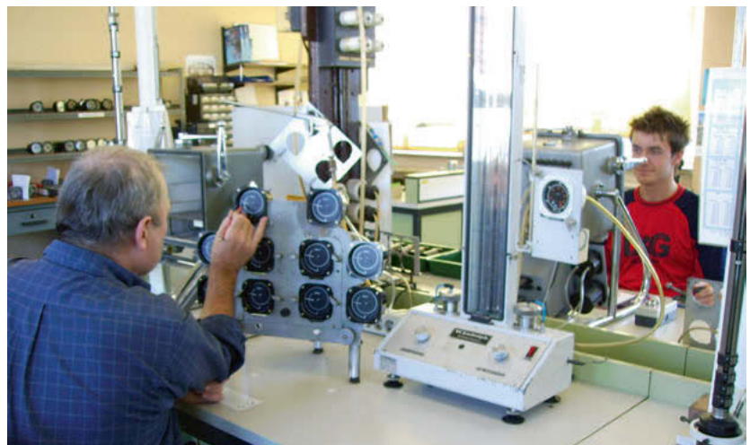
Left: production of spare part for diaphragms, and (above) calibration of airspeed indicators (All photographs courtesy of Winter Instruments)
