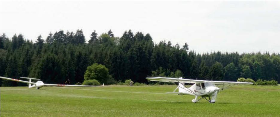
The Ikarus C42 is popular in Europe, particularly in Switzerland, with 125 in use as tugs at airfields at 2,000ft or more altitude and up to 700kg gliders
