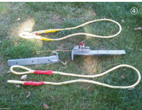
A collection of handling ropes, with bottom ground anchor and top 'ground Ottfur'
