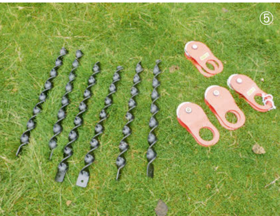
(Above left-right): 'groundbolts' and pulleys; 2 to 1 pulley autotow system; 3 to 1 pulley autotow system (Pete Whitehead)
