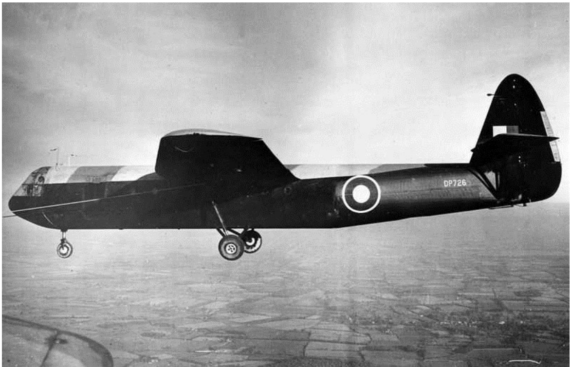
The British built Airspeed Horsa glider was made completely of wood, had a wingspan of 88 feet and was 67 feet long. The load capacity was 7,750lbs.
